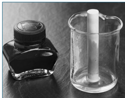
figure 12.5 This simple chalk chromatogram shows the separation of black ink into its different components.
