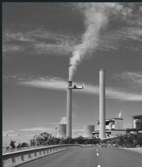
figure 12.1 Qualitative and quantitative tests are carried out on the air samples collected by the CSIRO plane near a coal-fired power station to monitor the gas emissions from the power station.
