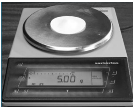
figure 13.2 An electronic balance is used to measure the mass of substances in gravimetric analysis.
