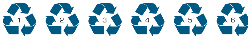
figure 10.18 These symbols indicate what type of polymer has been used in the item.
