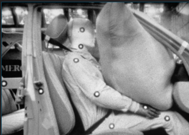
figure 15.1 The chemical reaction that inflates vehicle air bags must occur in milliseconds.
